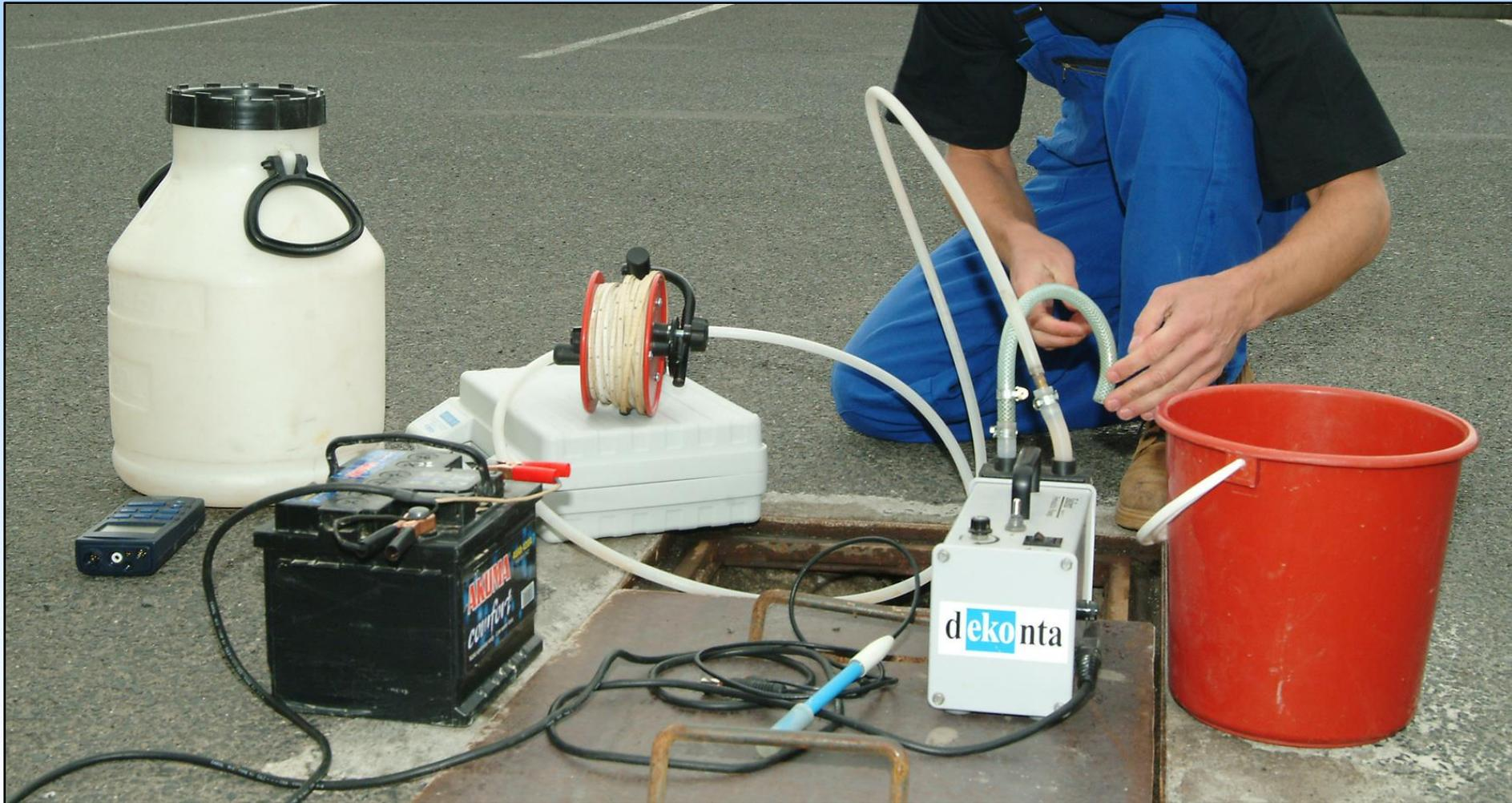
From the sampled well is pumped required amount of water, usually 3-5 volumes before sampling.
